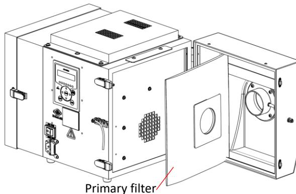
5. Install the new primary filter and install the secondary filter back in place.
