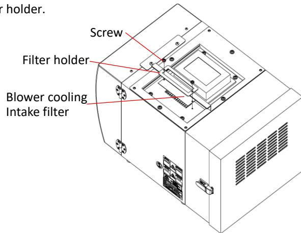
3. Install the new blower cooling intake filter and install the filter holder and secure it with two screws.
