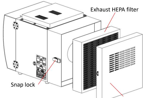
2. Remove the exhaust HEPA filter.
