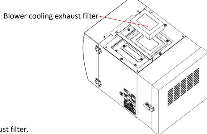
3. Install the new blower cooling exhaust filter.
