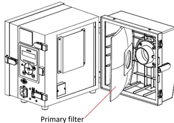
4. Install the new primary filter and install the secondary filter back in place.
