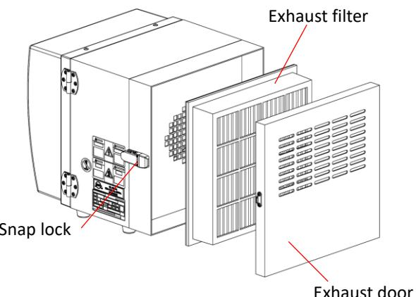
2. Remove the exhaust filter.
